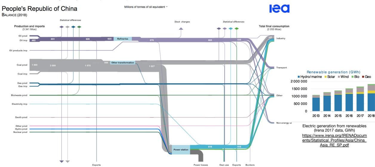
Primary energy supply depends largely on coal and oil, though RE and Gas is increasing. Final consumption mainly by industry, only 24% via electricity.
